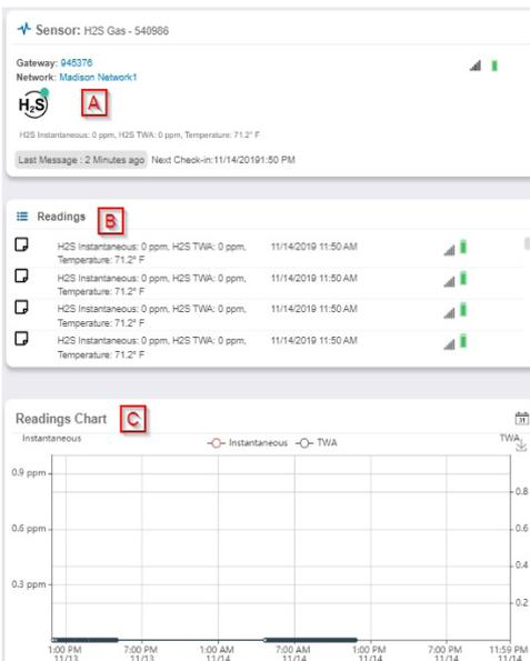
**A.** The sensor overview section will be above every page. This will consistently display the present reading, signal strength, battery level, and status.
